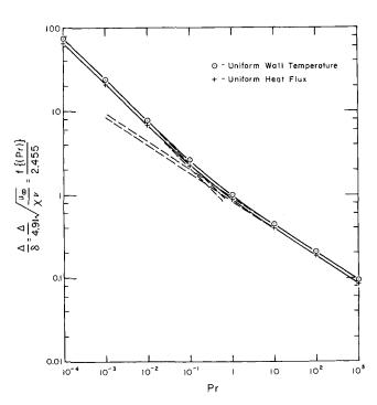
The curves in Figure 1 correspond to Equations (9) and (10). The equations rather than the graph are recommended for numerical work and for subsequent derivations involving the thermal boundary layer.
